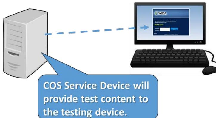
Central Office Services (COS) is a software tool that allows you to install, configure, and manage your online testing environment from a central location. Registering a testing device to a configuration defines which COS Service Device will provide test content to the testing device.
